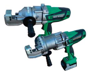
BATTERY POWERED REBAR CUTTERS will safely and cleanly cut rebar up to #5 (5/8") and #6 (3/4") GR-60 respectively. These self-contained electric/hydraulic units will also cut other items like chain, bolts, and rods.
