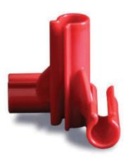
KODI KLIP Korner Klips provide for easier, faster, 3-way corner strengthening. They eliminate wracked, twisted, or out-of-alignment cages and baskets by rigidly enclosing corners with less rebar bending, no welding, and no double wire tying.
