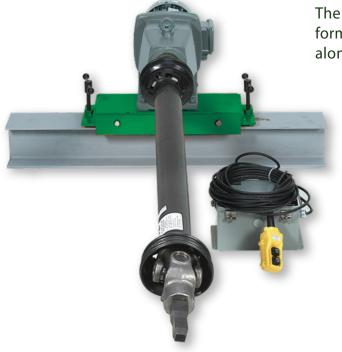
The GO-E2 is an electric-powered Gate Opener with a rotating platform (for a full 360° swivel) on a rolling carriage (to mount and slide along a secured-to-ground W-beam), utilizing pendant-controlled,
